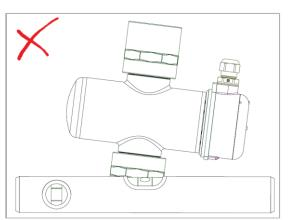
Incorrect vertical mounting, the lamp is not placed horizontally.
