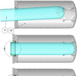
Remove the quartz tube (11) from the packaging and carefully check it for damage. Damaged quartz tubes cannot be used due to the risk of leakage and / or short circuit.
