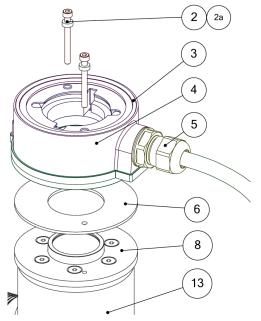
Ensure that the O-ring (3) is not lost. Tip: store it temporarily. Insert both M4x45 screws (2) with the spacers (2a) around them in the holes of the lamp socket. Place the foam gasket (6) at the ends of the screws so that it can be placed as a whole on the mounting flange.
