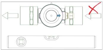
Incorrect mounting of the lamp holder, the arrow on the lamp base must point with the direction of flow and not as shown here against the direction of flow.
