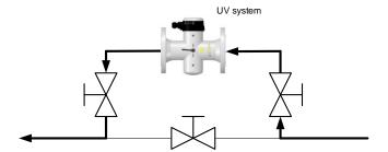
Bypass closed for UV system operation
