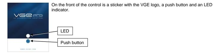
If the UV system is switched on, the program will check itself. The LED will flash red rapidly for approximately 1 second. After this the LED lights up green, blinks green or lights up red. This depends on the number of hours that the system has already been in operation.
