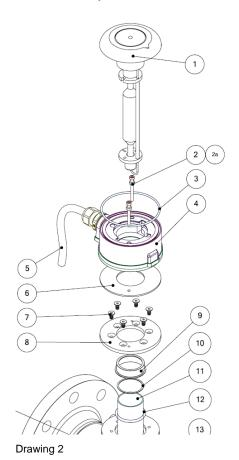
The lamp socket (4) is the electrical connection between the lamp and the lamp driver. It also plays an important role in the positioning and temperature management of the lamp. The lamp socket is mounted onto the mounting flange (8) by two screws and plastic spacers (2, 2a). The mounting holes are symmetrically positioned on the mounting flange, allowing the lamp socket to be mounted in two ways. In other words the socket can be rotated 180°.
