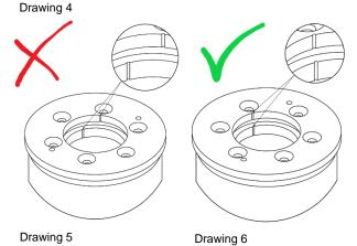
The mounting flange (8) can now be positioned with respect to the hole pattern on the irradiation chamber (13). The mounting flange can only be positioned in one way. To simplify correct positioning, markings have been applied to the irradiation chamber and to the mounting flange. (see drawings 5 and 6) When the markings are in line, the holes correspond.
