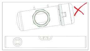
Incorrect horizontal mounting, the lamp is not placed horizontally.
